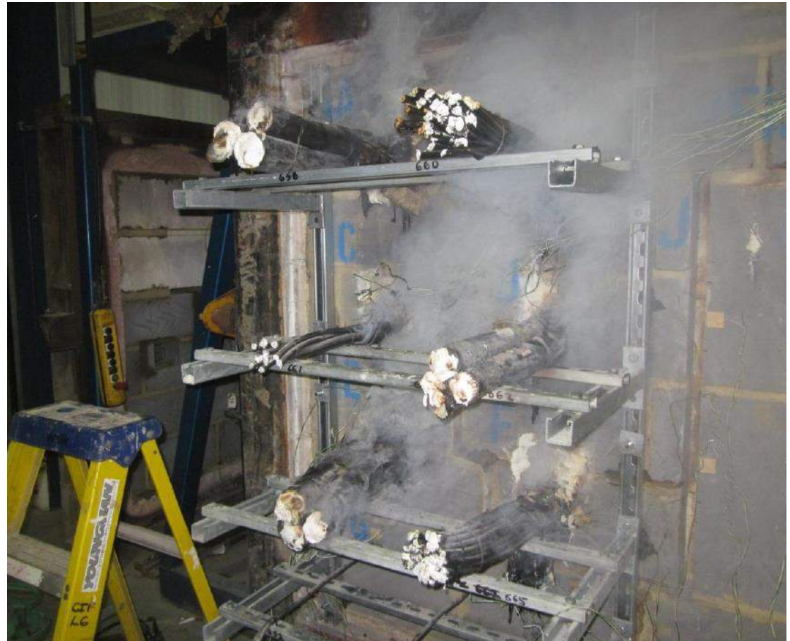
Photo shows a fire test after 2 hours at Warringtonfire in UK
